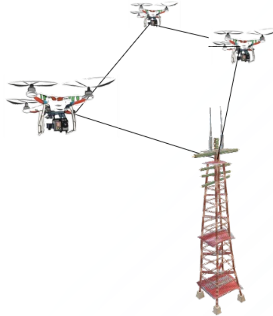
NLoS communications through ground infrastructure
